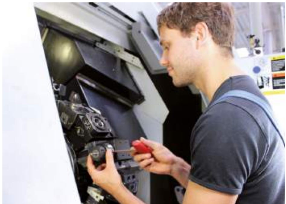
Tool Change for a driven tool with BENZ Solidfix® on the CNC turret. Above: Right Angle tool with BENZ CAPTO™ interface
