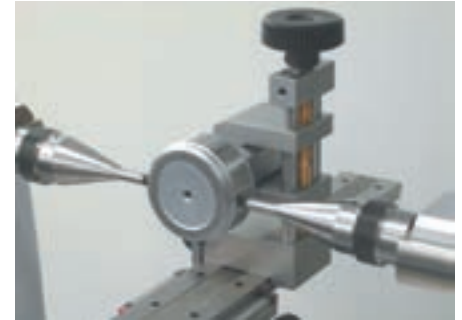
Plug gauges / pins without centers up to dia. 100mm
