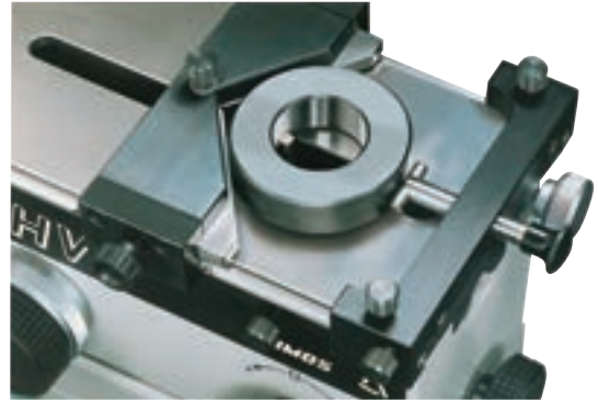
4) Checking of internal diameters
