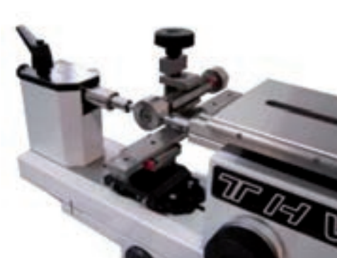
3) Checking of plain and threaded plug gauges using the floating table
