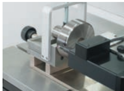
Checking of taper thread gauges (plug/ring gauges)
