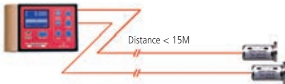
ZEROTRONIC sensors connected to a BlueMETER
