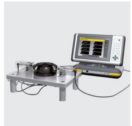
Capacitive probes on a jig
