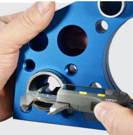
Deep measurement with S_Cal EVO Smart DM
