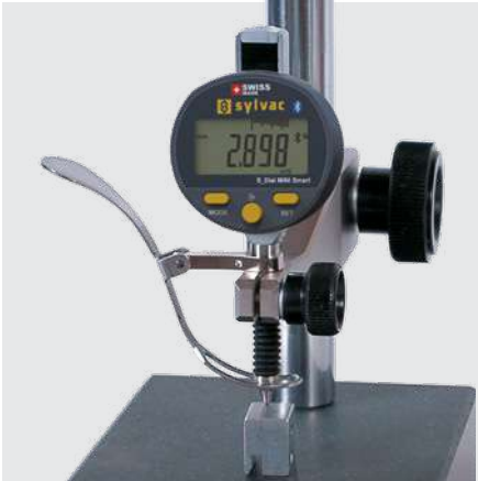
Lower lifting lever, type 905-4214
