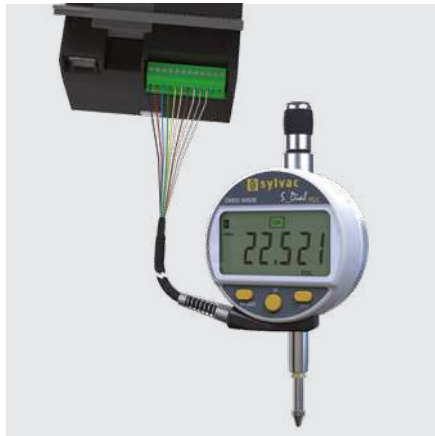
S_Dial WORK PLC connected to a PLC
