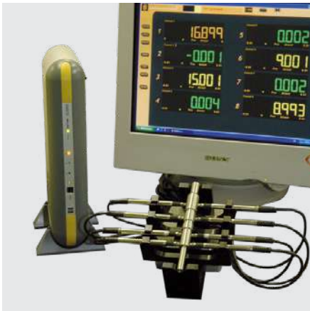
Dynamic measurement of several diameters, (OD and ID) of a shaft
