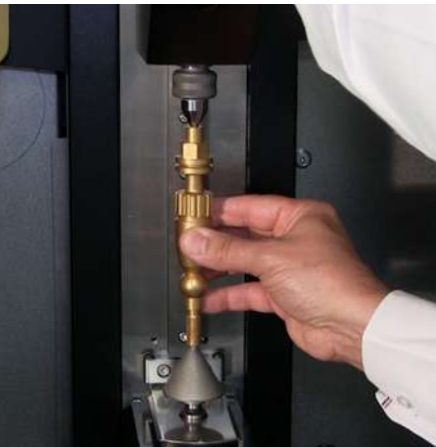
Part measurement with SCAN F60
