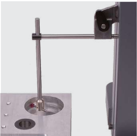
Internal groove measurement with accessories 930-2108, 930-2110 and 905-2207
