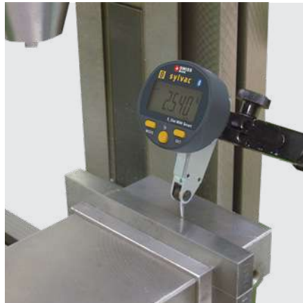
Checking the alignment on milling machine.
