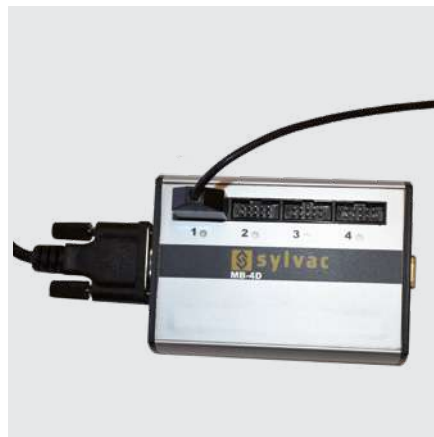
Digimatic instruments connected to a MB-4D
