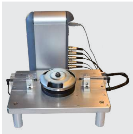
Capacitive probes connected to a D200S
