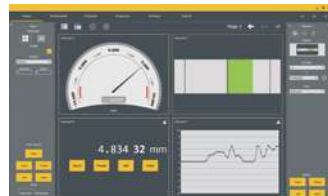
Multi-channel display with colour-coded tolerances
