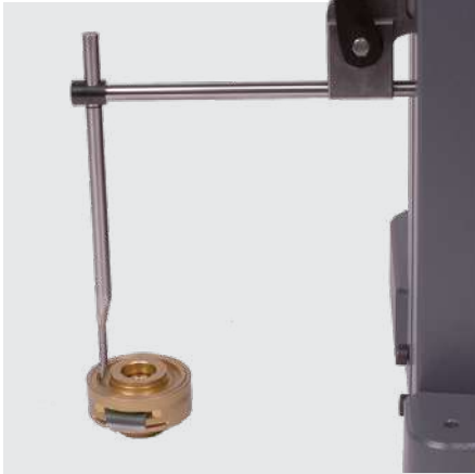
Depth measurement with accessories 930-2108 and 930-2105
