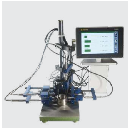
Inductive probes connection on a jig
