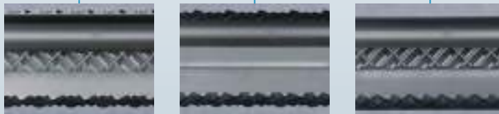
Cross tothing, upcut Finishing cut Cross tothing, downcut
