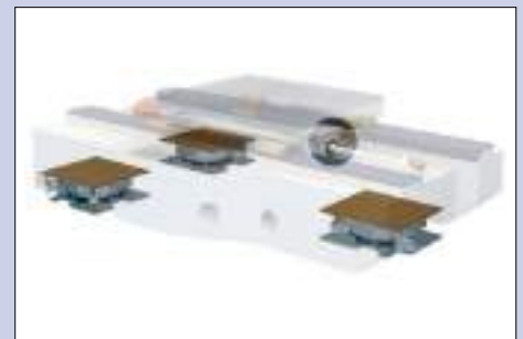
Actively controlled, integrated, vibration damping measuring table.
