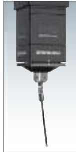
SurfaceMeasure probe scanning a complex surface.
