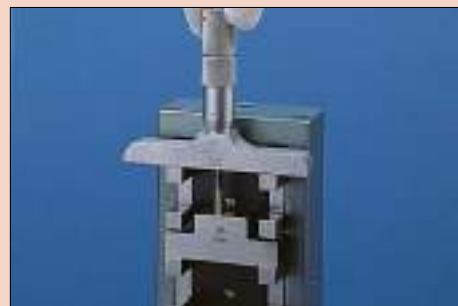
A 25 mm anvil block provides the reference surface for the depth micrometer rod.
