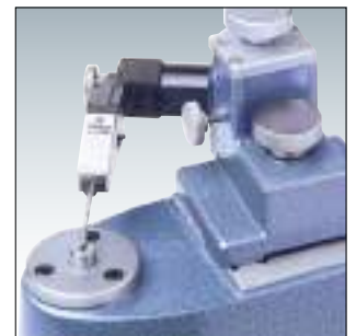
Calibrating a lever probe head.
