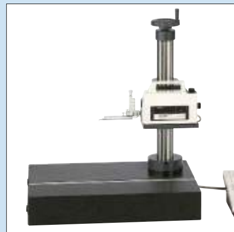
The SJ-500 can also be mounted on a manual column stand.
