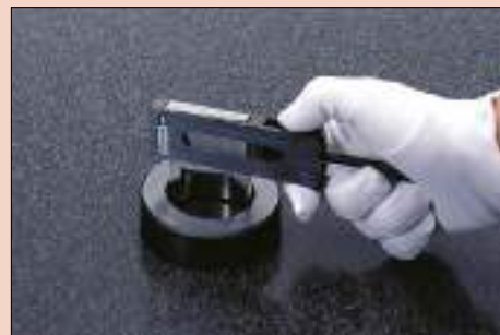
Gauging a bore using a pair of half round jaws and a holder.
