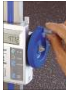
Slider height adjustment wheel.
