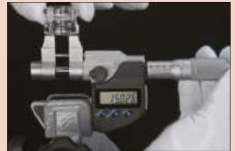
Measuring a small inside diameter.
