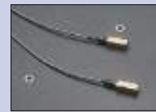
Workpiece thermal compensation system temperature sensors.
