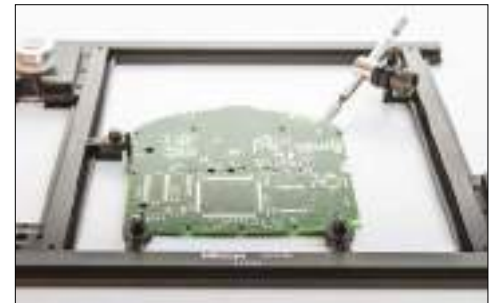
Support and clamping of a PCB at three points to enable positive location of the irregular profile at the measurement position.
