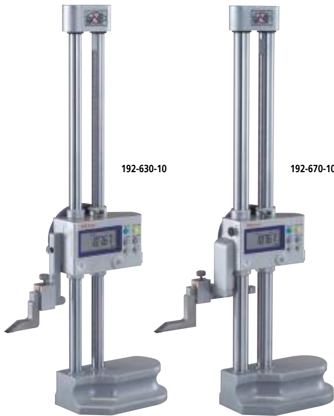
Offset height adjustment wheel improves ergonomics.
