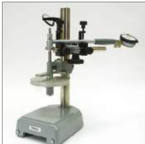
Calibrating a bore gauge.
