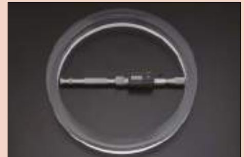
Using a setting ring to accurately set an inside micrometer.
