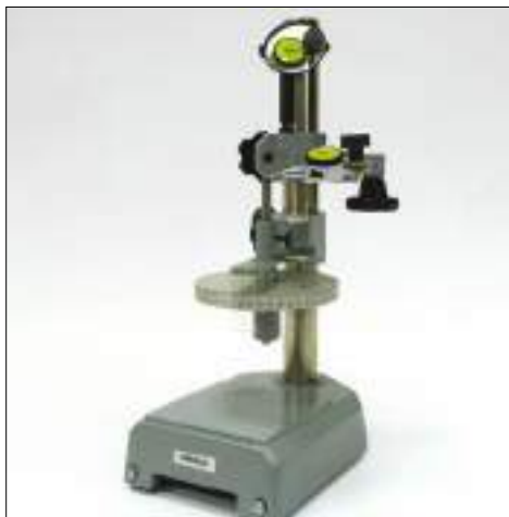
Calibrating a lever indicator.
