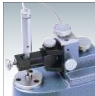
Calibrating a probe head.
