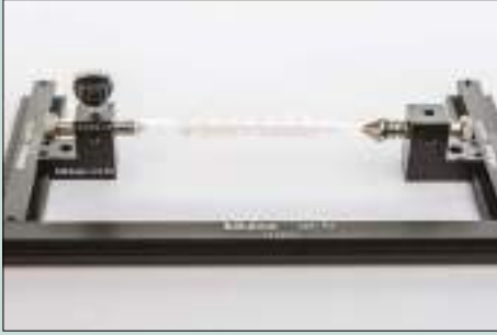
Holding a cylindrical part between centres.
