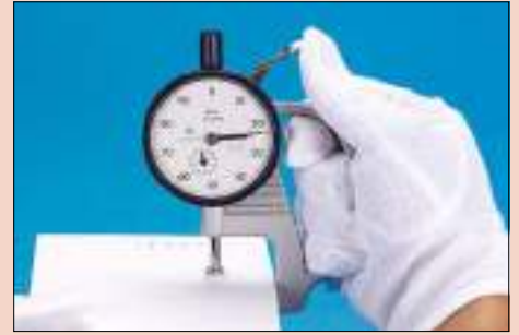
Measuring paper thickness.
