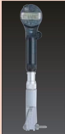
ABSOLUTE Digimatic Bore Gauges, which integrate the display with a bore gauge measuring unit, are also available.
