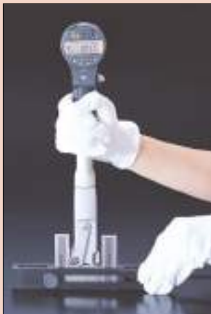
Setting the Bore Gauge to a master value using a gauge block set.
