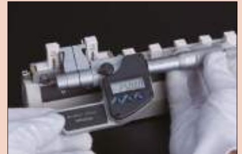
Using an Inside Micro Checker to accurately set an inside micrometer.
