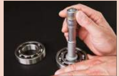
Ball-bearing inner-race inside diameter measurement.
