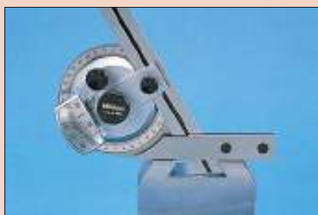
Measuring an internal dovetail slide angle.
