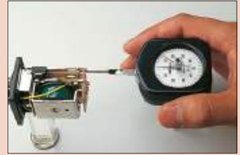
Measuring contact force on a relay.
