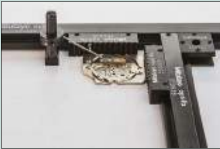
Toothed location elements provide access to edges for the camera while one or more spring clips lightly clamp a part in the measurement position.
