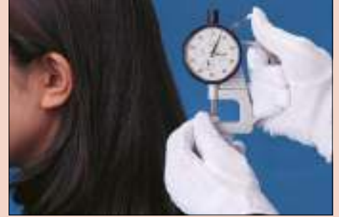
Measuring thickness of a human hair.
