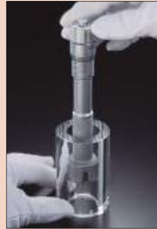
Constant-force device ensures repeatable measurement.
