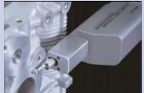
SURFTEST probe measuring surface roughness.
