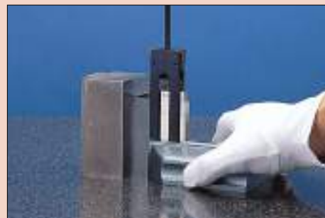
Marking a workpiece using the base, a holder and the scribe point.
