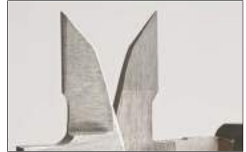
Carbide-tipped jaws for inside measurement.
