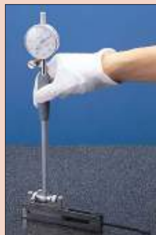
Setting a bore gauge using a holder with the pair of Type I half-round jaws arranged as flat contact surfaces.
