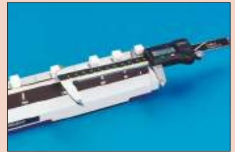
Checking the accuracy of a caliper (inside measurement).
