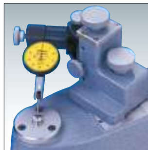
Calibrating a lever indicator (dial test indicator).
