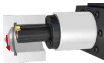
3 Cutter lifts from workpiece
