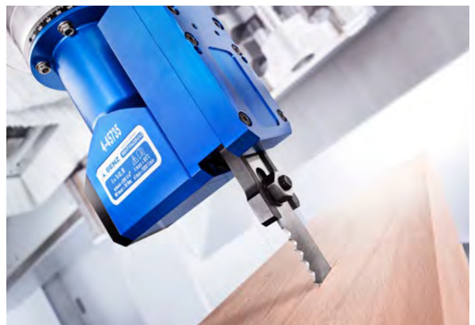
Vertical insertion of slots for fiche hinges
