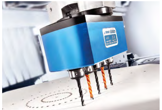
Drill rows in acoustic boards
