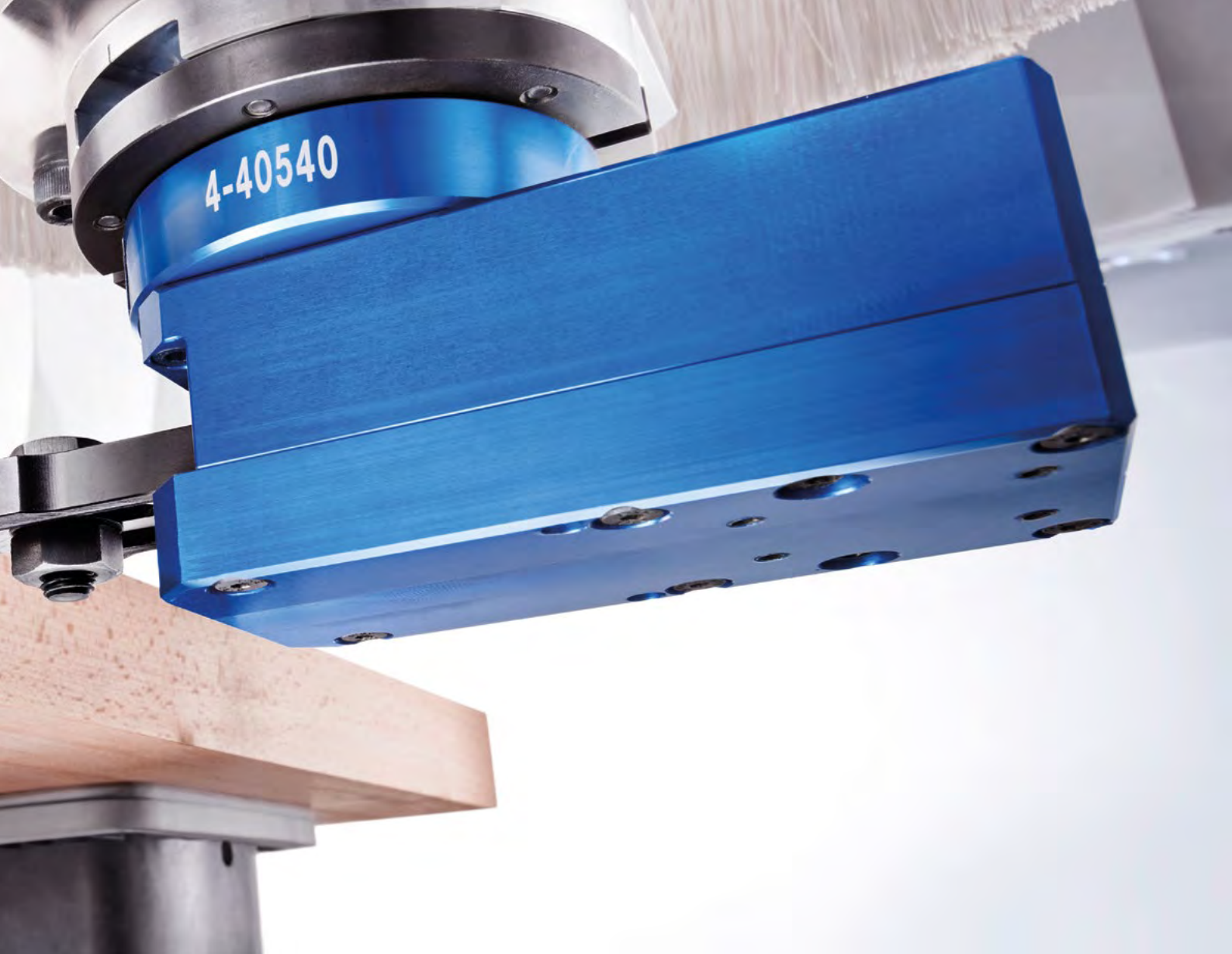
Horizontal insertion of slots for fiche hinges
