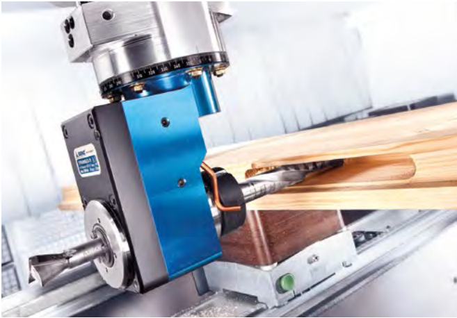
Milling lock cases and faceplates
