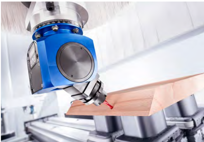
Dowel drill holes in miter
