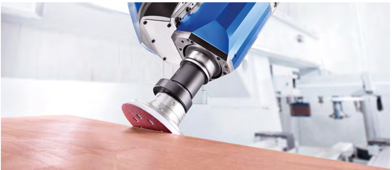
Chamfer sanding on a step
