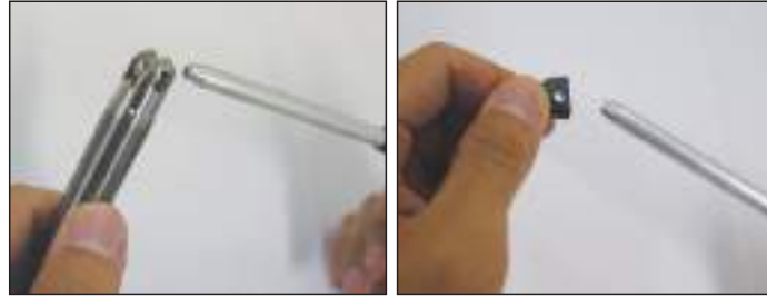
▲ Make sure to clean the insert and insert seat
