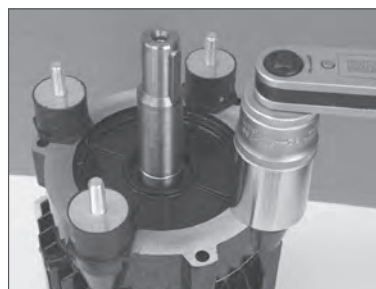
(11) Remove old motor mounts and replace with new mounts. Tighten mounts to 8Nm on S Series, 10Nm on FX Series.
