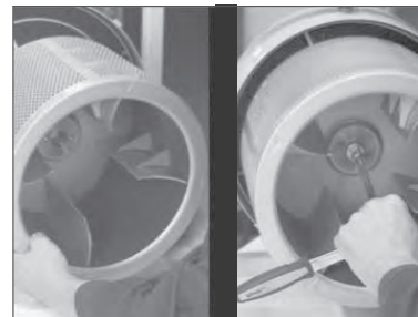
(15) On the S Series, ensure bush, shaft and drum hub are clean and free from debris before re-fitting drum. Tighten drum bush to 20Nm. On FX Series tighten drum bolt to 8Nm.
