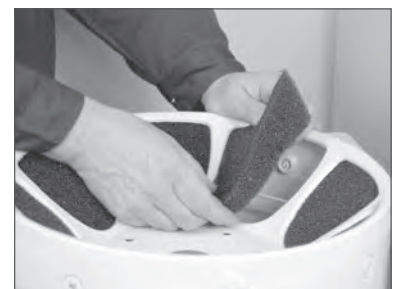
(12) Remove old silencer & fit new silencer.
