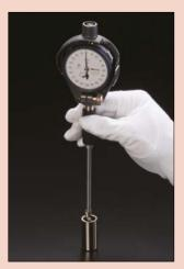
A heatshield prevents accuracy degradation due to hand heat during prolonged use.
