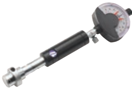
SmartPlug with depth stop
